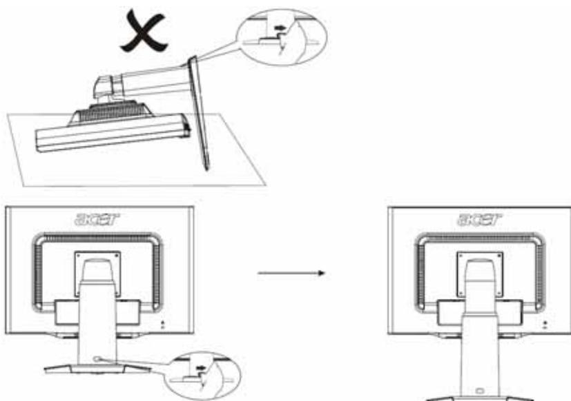
Slide the lock to right from the display support frame as per the figure and then adjust the height. Note that to slide the lock to right, erect the machine on the table to prevent the top part of the display from ejecting.
