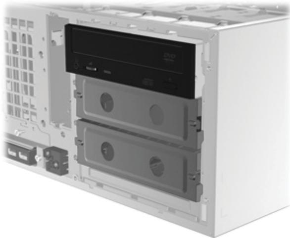
9. Replace the front bezel and the side access panel when finished.
