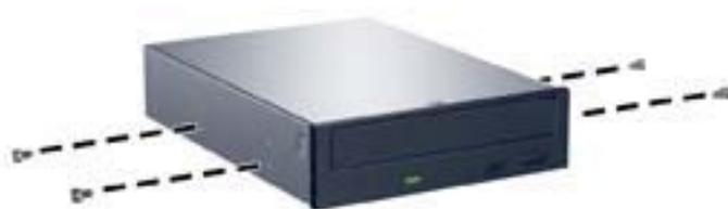
5. Position the guide screws on the drive into the J-slots in the drive bay. Then slide the drive toward the front of the computer until it locks into place.
