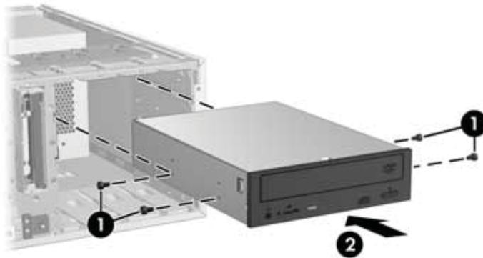
4. Align the screws with the grooves in the drive bay and gently slide the drive into the bay until it snaps into place (2).
