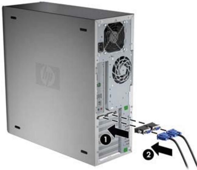
2. Connect the other ends of the graphics cables to the monitors as shown below.
