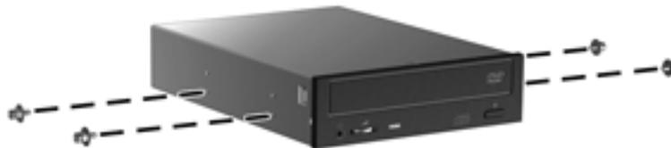
4. Align the screws with the grooves in the drive bay and gently slide the drive into the casing. Slide the drive completely in until it snaps into place.
