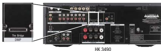
Figure 20 – The Bridge II Connection
