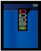
When the battery is low, the display will flash a message to remind you to charge the battery.
