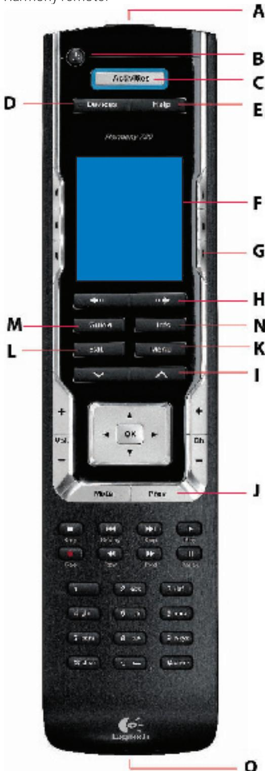
**A.** USB Connector: Connect one end of the USB cable to this connector and the other end to your computer so that you can download your configuration using the Harmony remote software.
