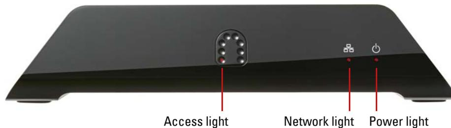
The Access light glows when you are connected to your Slingbox, either at home or remotely. The Network light glows when your Slingbox is communicating with your home network. The Power light glows when your Slingbox is connected to power.
